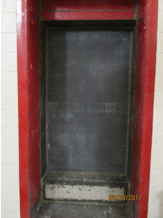
Figure 1 – Specimen mounted in the test opening.
