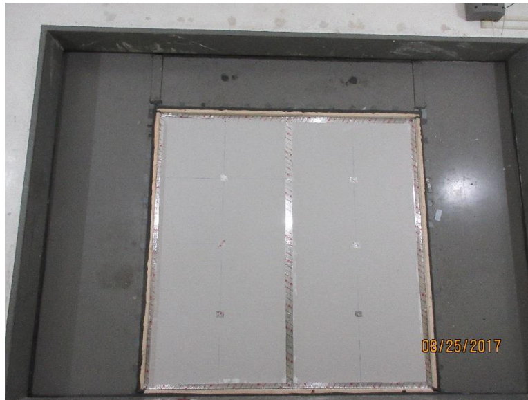
Photo No. 3 Source Room View of Installed Specimen
